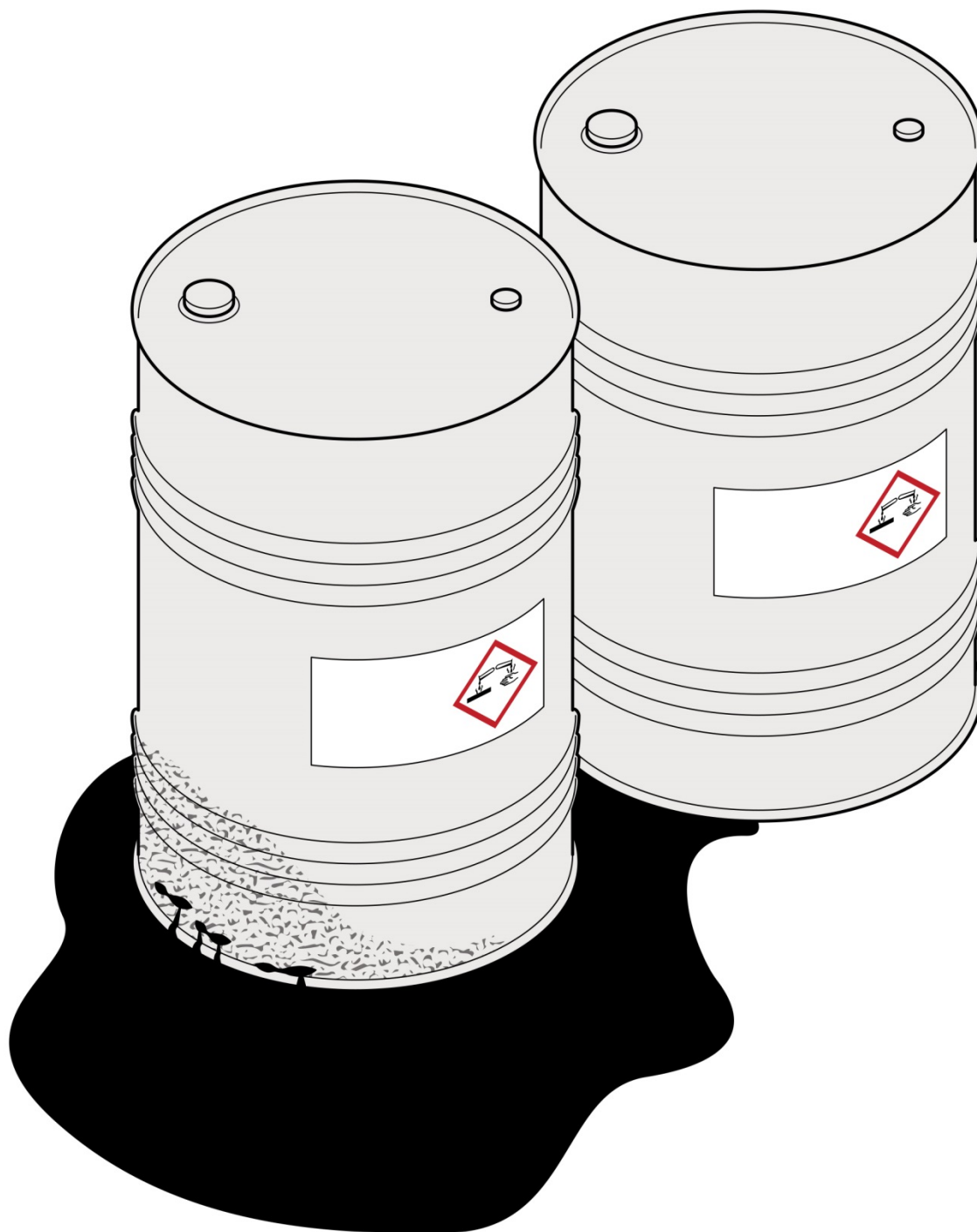
Figure 7 Chemical stores should be inspected regularly to prevent spills and other incidents
